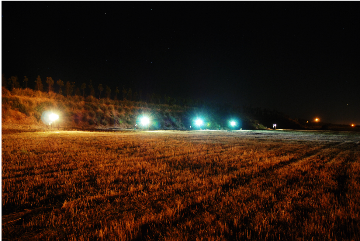
PLATE 1. Image showing one experimental block with five of the six different color temperature LEDs. Note the dark spot between the 4th and 5th light as the location of the just visible control treatment. The 6th color temperature is not visible and is to the left of the image. Individual lights were placed 20 m apart with different blocks placed 200 m apart. Photo credit: S. M. Pawson, Scion.
