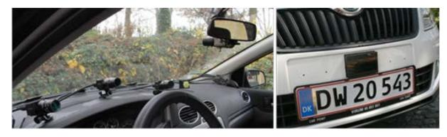
Figure 1: The 3-camera system for tracking eye movements together with the scene camera behind the rear view mirror (photo left). The scanner is installed in front of the car (photo right).
