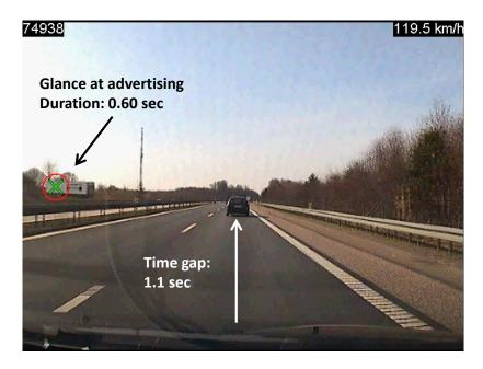
Figure 3: Safety buffer =  $Time\ gap\ to\ vehicle\ ahead\ (seconds)\ minus\ advertising\ glance\ duration\ (seconds).$
