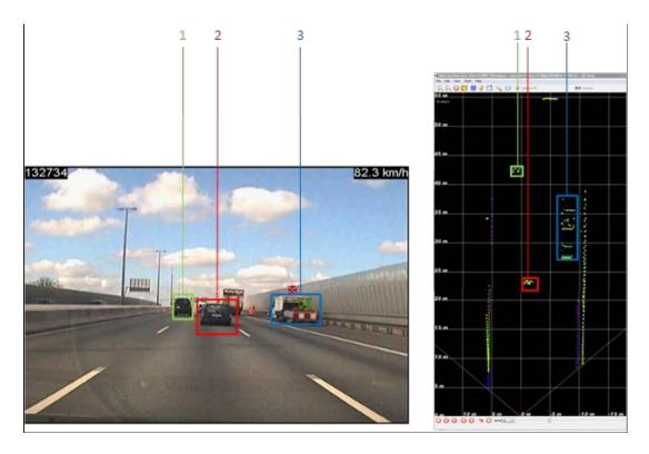
Figure 2: Example. Screen dump photo from the scene camera (left) and the laser scan result (right) from the same traffic situation. The small green cross with the red ring around it on the photo indicates the eye glance direction of the test driver.
