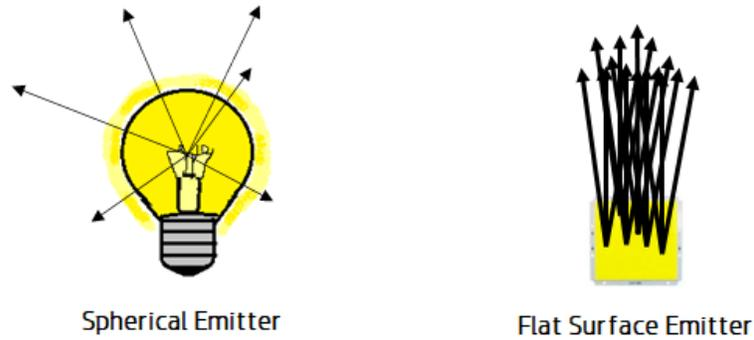
Figure 1 - Spherical vs. Flat Surface Emitter
