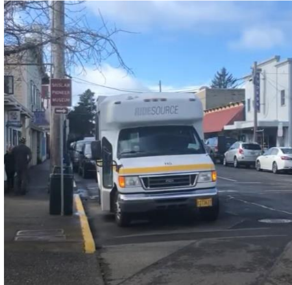
Figure 10 - Non-LED Hazard Lights
