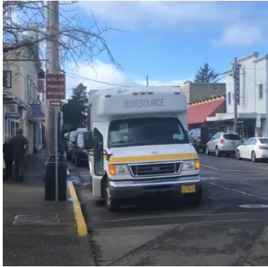
Figure 8 - Non-LED Hazard Lights
