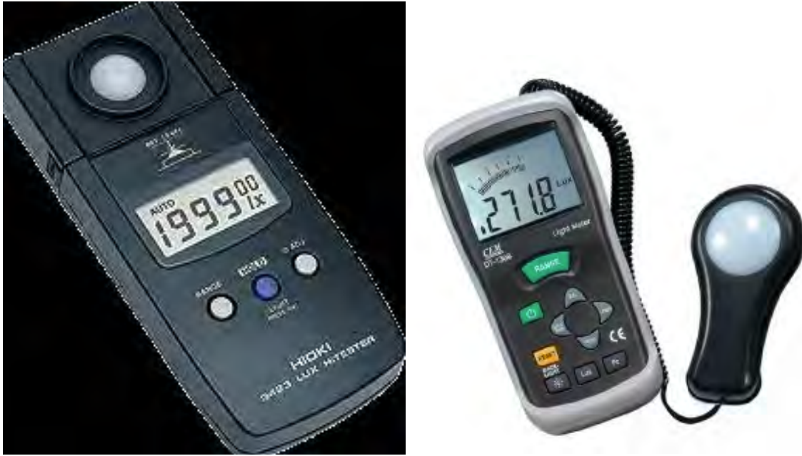
Figure 2: Two Typical Illuminance Meters Each displays a reading in Lux (lx) (Note the white “dome” that collects light, and the lack of a viewfinder)
