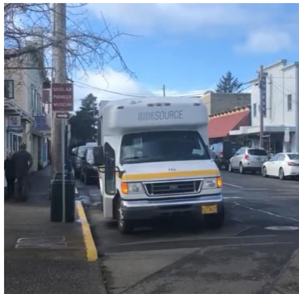
Figure 11 - Non-LED Hazard Lights
