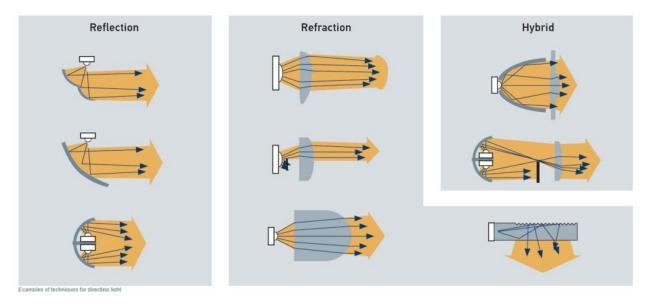
Figure 26 - Optics Diagram of LED Headlight
