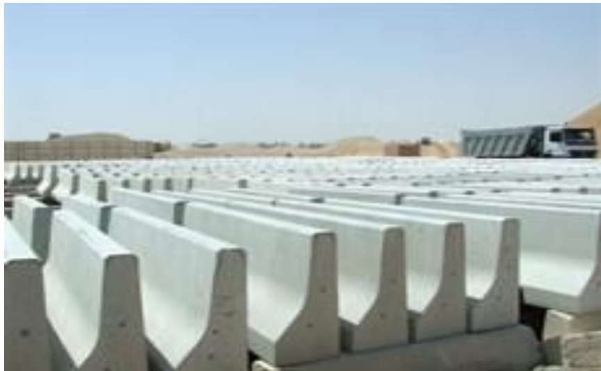
Fig 6: Concrete baffles intended for use on a motorway in Egypt. Credit: World Highways. http://www.worldhighways.com/categories/road-markings-barriers-workzone-protection/features/safety-barriers-deliver-valuable-road-user-protection/
