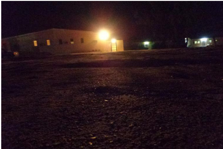
Fig 3: Glare, caused by inappropriate lighting. The unshielded light located on the gable end of this house was installed to enable worshippers attend a local mosque. Complaints had been made that they couldn't find their way to attend the Maghrib, Ayesha and Fajr prayers that occur during the hours of darkness. In fact the situation became worse as anyone approaching the light was dazzled to the point that he could hardly see the ground beneath his feet. The light was never necessary and the problem could easily have been solved simply by asking worshippers to use a torch. Image: C. Henshaw.
