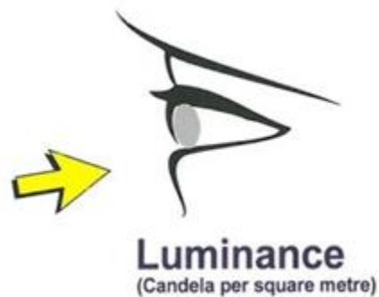
Figure 9 - Luminance is measured in candela per square meter or nit 22
