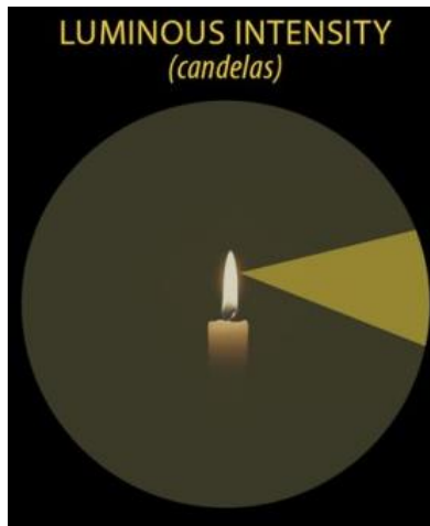
Figure 7 - Luminous Intensity is measured in one solid angle in candelas. 19
