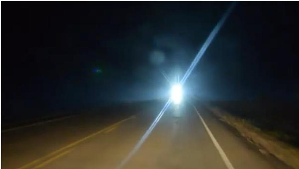
Figure 17 - LED Headlight Glare
