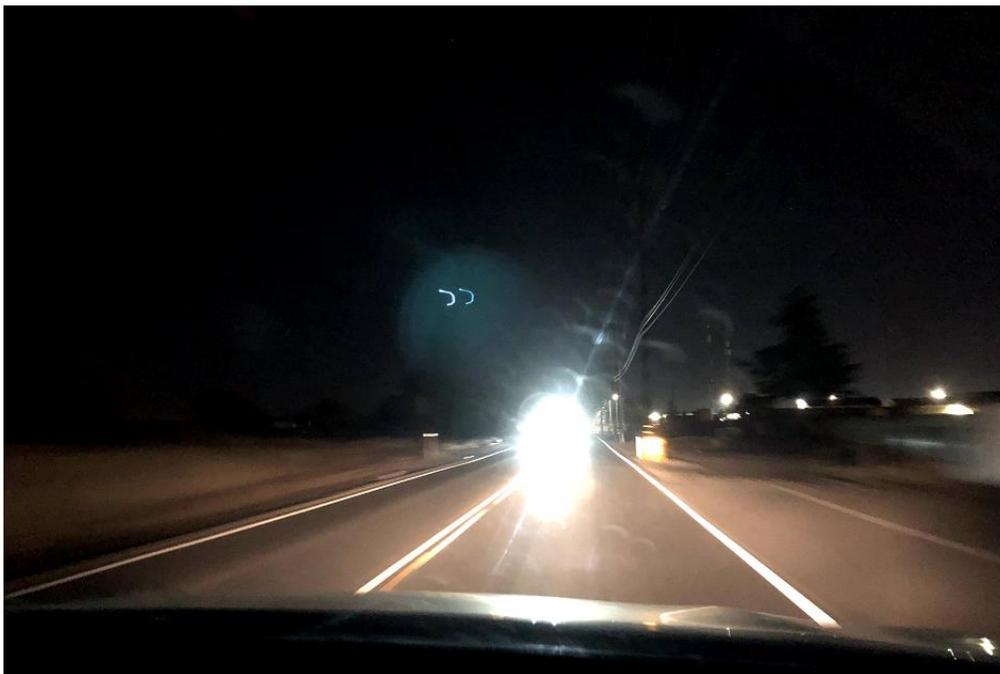
Figure 27 – LED Headlight Glare
