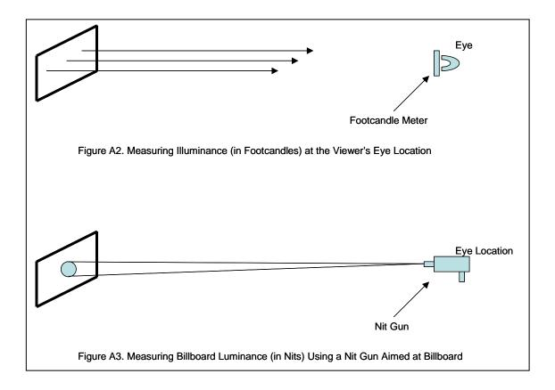
L, the billboard luminance, can also be measured with a "nit gun", which is a luminance meter that can be pointed at the billboard. Figure A3. However such devices are more expensive and less readily available than a footcandle meter.
