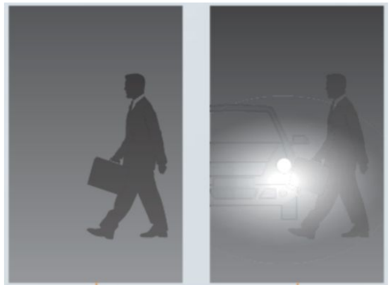
> Figure 8, a visual representation of veiling luminance caused by disability glare. Note how the contrast between the pedestrian and background is reduced.
