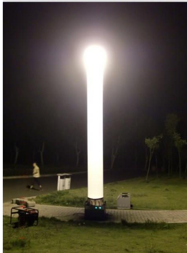
4 5 6 7 8 9 10 11 12 13 14 15 Figure 23 - Inflatable Tower Light
