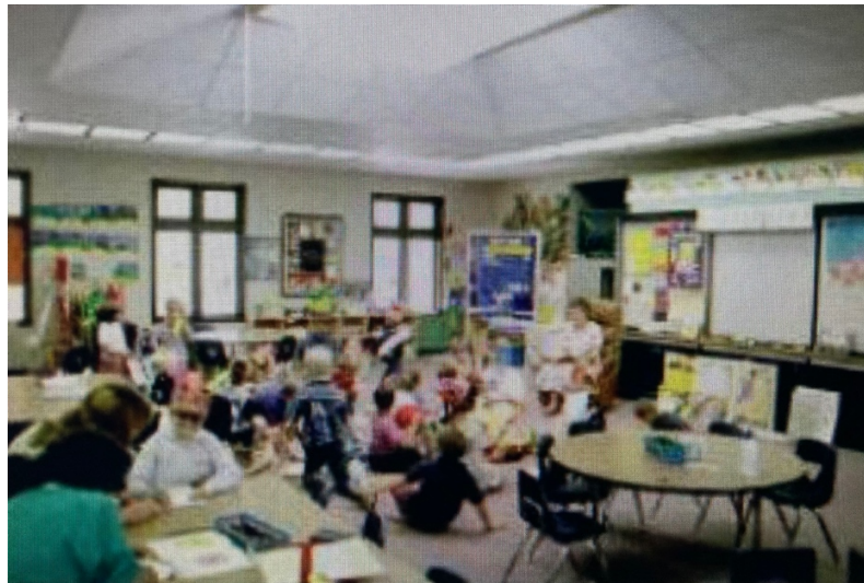
Classroom lit by skylight possessing a diffusing lens. Note how the light is spread evenly throughout the classroom.
