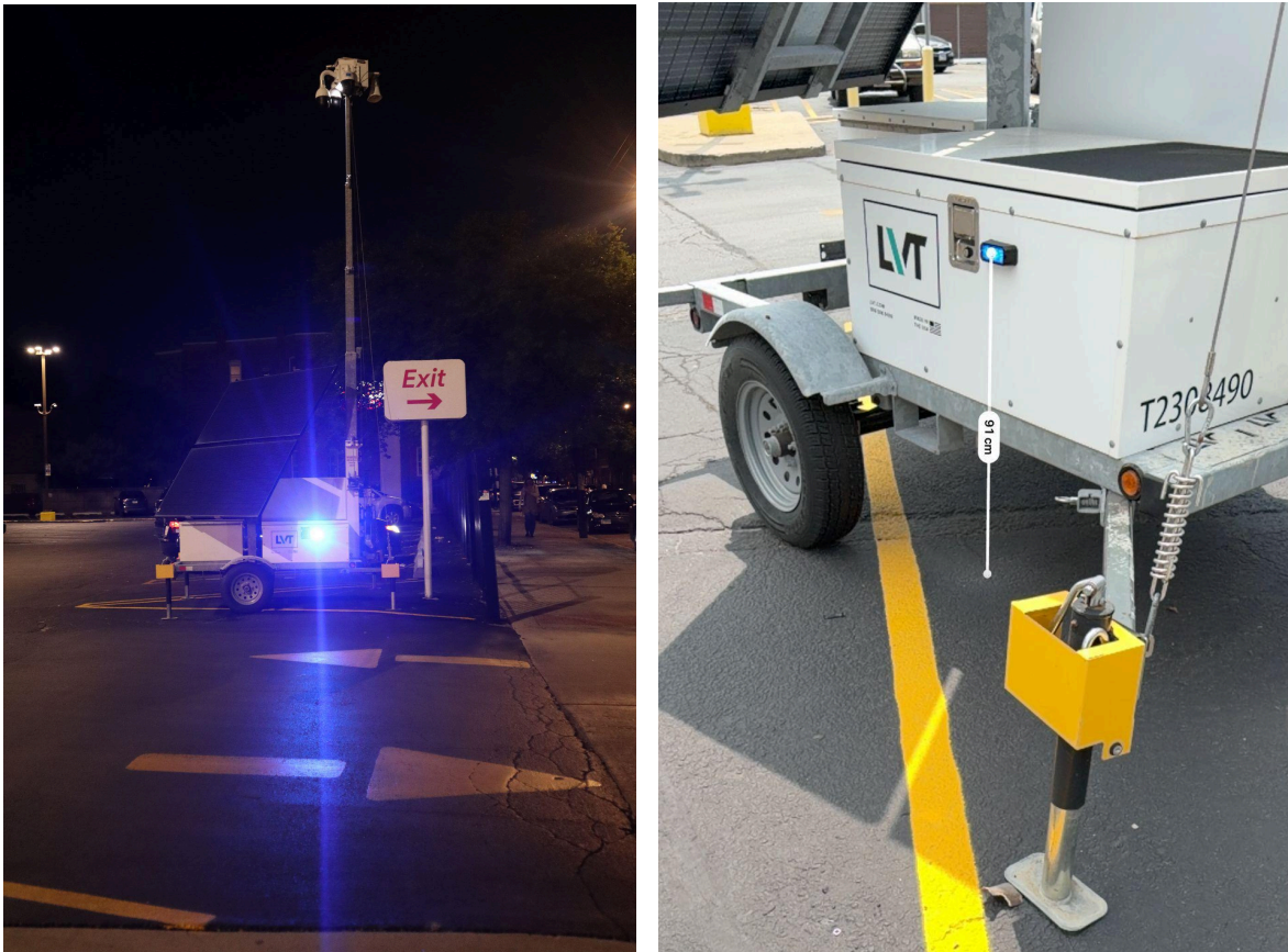
Figure 4: MSU unit lighting on main unit and mast (left) and height of main unit strobe above ground level (right) just below eye level.
