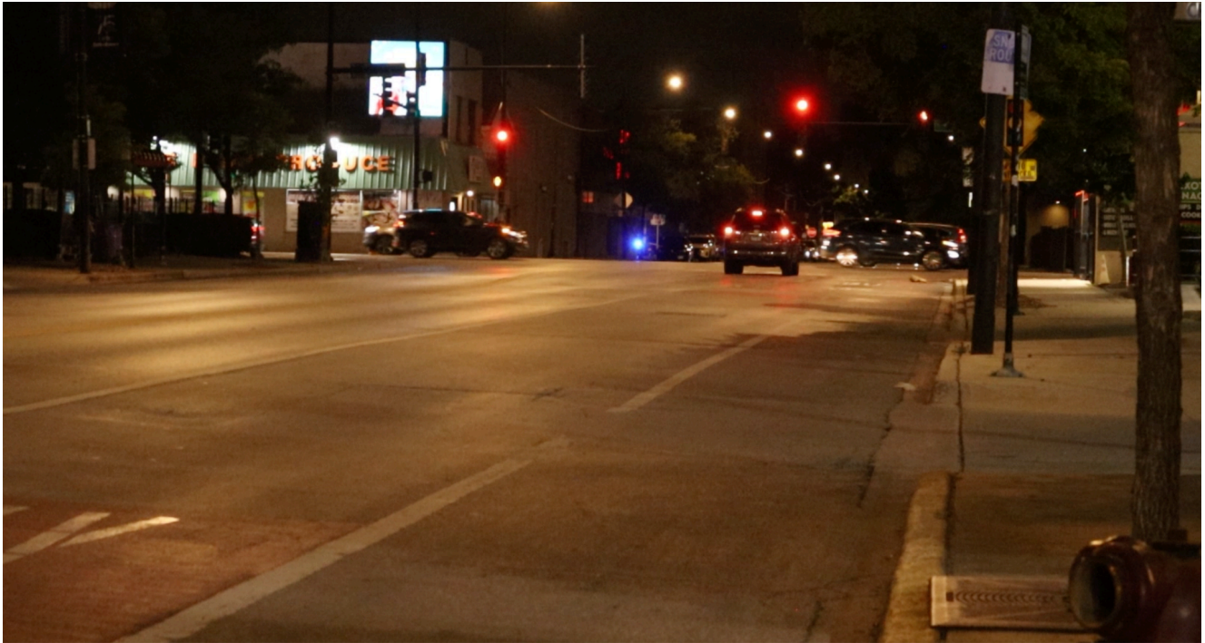
Figure 6: Blue Strobe Light (center) clearly visible from the roadway at a distance of more than 200m from the LVT MSU in the CVS pharmacy parking lot. Even from this distance it was visibly brighter than approaching headlights and street lights in view.
